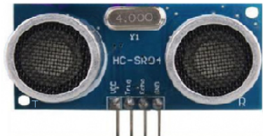
Vcc Trig Echo GND HC-SR04 Pinout
