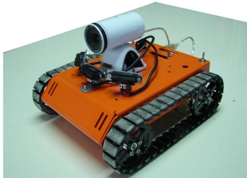
**Fig. 6.** ExaBot with 3 infrared telemeters and webam mounted
