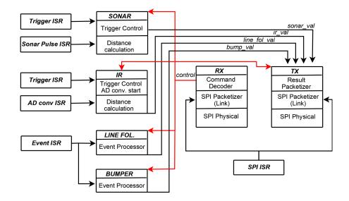
Fig. 3. PIC18F4680 Software Architecture
