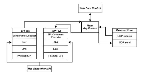
Fig. 5. PC104 Software Architecture
