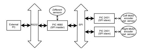
Fig. 2. ExaBot architecture without the PC104
