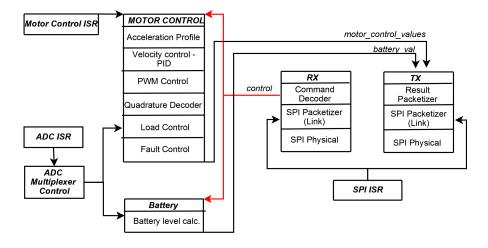
Fig. 4. PIC18F2431 Software Architecture
