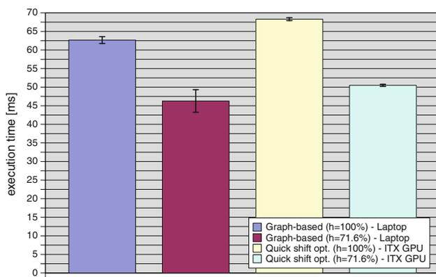
**(a)** Optimal choices of segmentation algorithm and executing platform
