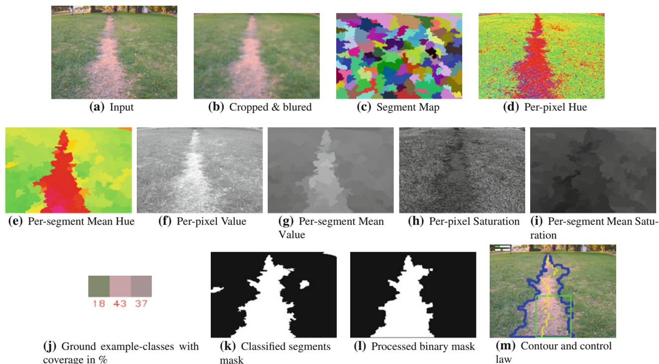
**Fig. 2** Pipeline description of the complete road-detection method: **a** input image as acquired from the camera, **b** cropped image below automatically detected horizon, **c** segment map. For each segment, mean and covariance are computed: **e**, **i**, **g** per-segment hue,
