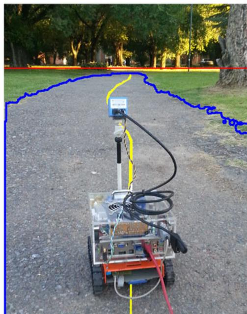
**Fig. 1** ExaBot robot performing autonomous navigation in an unknown outdoor environment. The horizon line (red) is detected as well as contour of navigable space (blue). Middle points of the road are computed (yellow) to guide the robot. To achieve real-time constraints imposed by robot motion, the image segmentation is implemented on a low-power embedded GPU (on top of the robot)
