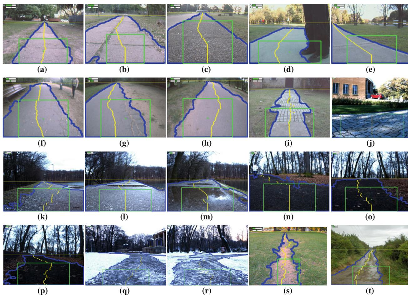
**Fig. 4** Example final images processed offline, as obtained from several datasets: the *green rectangle* represents the ROI used for extracting road appearance samples, the *yellow line* corresponds to the automatically detected horizon, the *blue contour* delimitates the
