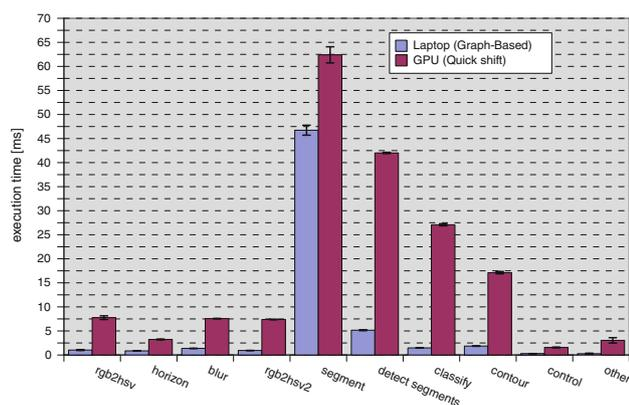
**Fig. 8** Absolute execution time for each step of the algorithm, in both platforms
