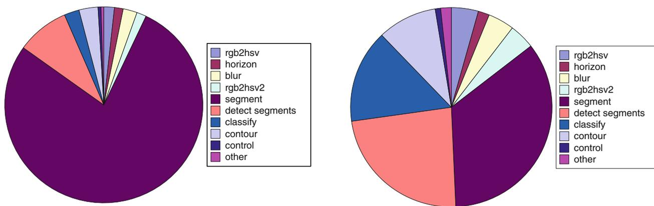
(a) Computation time of algorithm as executed on the Core i5 processor present on the Laptop
