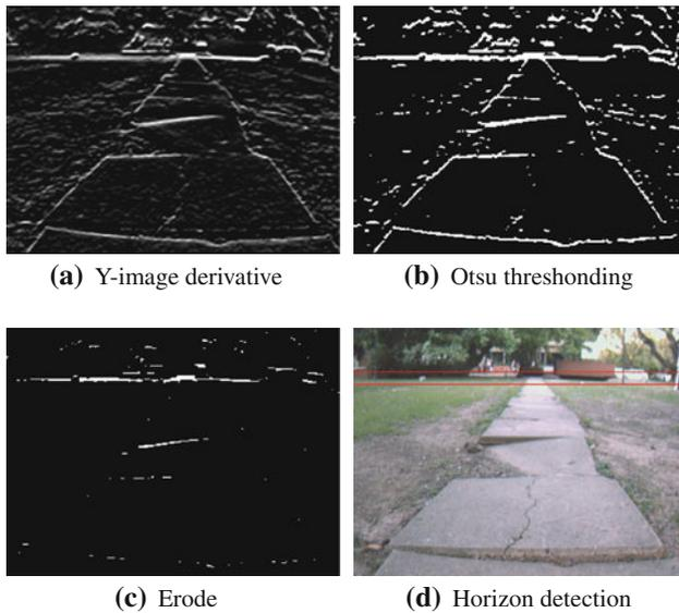
**Fig. 3** Pipeline description of the horizon detection algorithm: **a** Sobel operator is first applied to the input image to obtain  $Y$ -image derivative, **b** Otsu thresholding is used to transform  $Y$ -image derivative to binary, **c** an erosion filter is applied to reduce noise and remove thin lines, **d** a histogram is computed to find the sub-image where the horizon line is located
