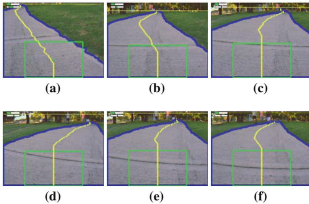
**Fig. 5** Example of online testing: series of successive frames where robot was started from a deviated position and ended with robot centered in road
